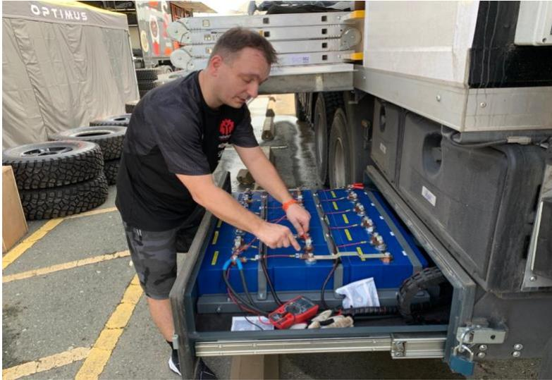
In the field, the batteries have proven themselves as very reliable, driven by competitor Jan Tomanek's Tatra. "We didn't dismantle them until Jan finished. Helping Ales Loprais on the track was his primary role, driving the support vehicle. He confirmed the batteries work perfectly and are functional after three demanding stages. The voltage only dropped a meager 0.02 volts in the full thirty days they spent in the car. This confirms the assumption that even racing trucks can be electric.
